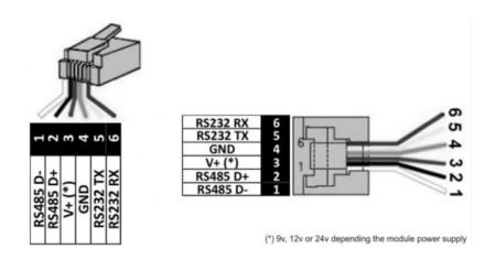
IMPORTANT when using the RS485 connector provided by Wattics:
