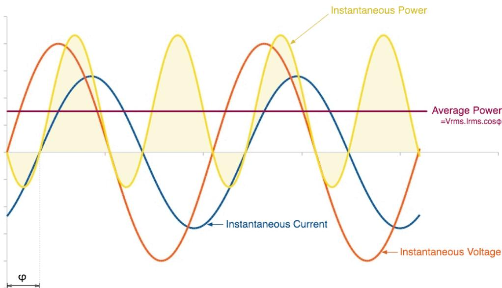
Power is the rate at which energy is consumed by an electrical load or produced by a generator, and the value of instantaneous power is obtained by multiplying instantaneous voltage with instantaneous current.
